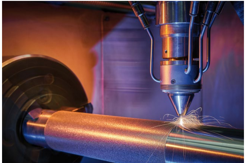
Fig. 1 Using EHLA to coat a piston rod (Source: Fraunhofer ILT / Volker Lannert)
