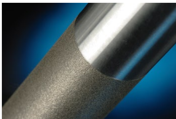
Fig. 6 EHLA coated and partially post machined piston rod (Source: Fraunhofer ILT)
